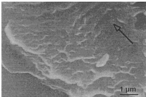
Figure 9 Side view of a liquid-nitrogen fractured film processed with a 20/80 MEK- n -decane (5 min soaking) and dried in the air. Arrow direction is perpendicular to the surface of the film.
